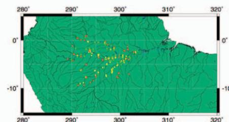
Figure 1 Amazon grading for ERS2 timeseries against nearest gauge data: green good, yellow moderate, red poor
