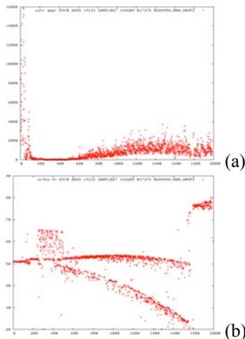
Figure 7 Waveform amplitude (a) and height (b) for location B plotted against echo number
