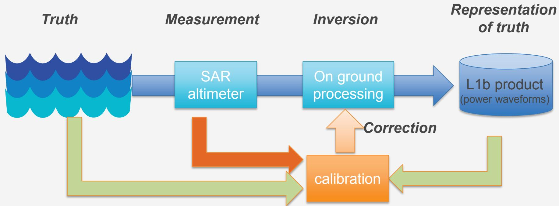
*The calibration introduces a correction feedback to reach the required quality of the data*
