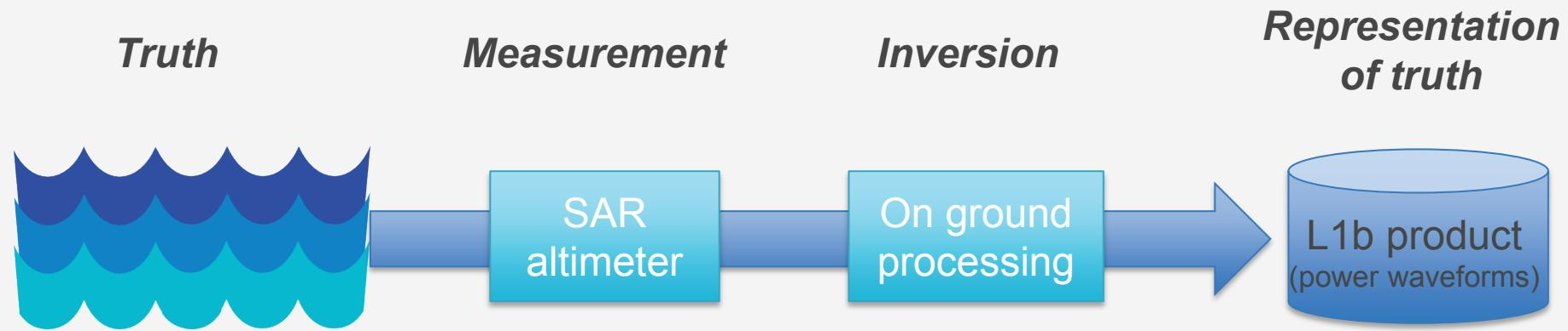
*The power waveforms are affected by any distortion introduced by the acquisition, unless that these distortion are properly compensated*
