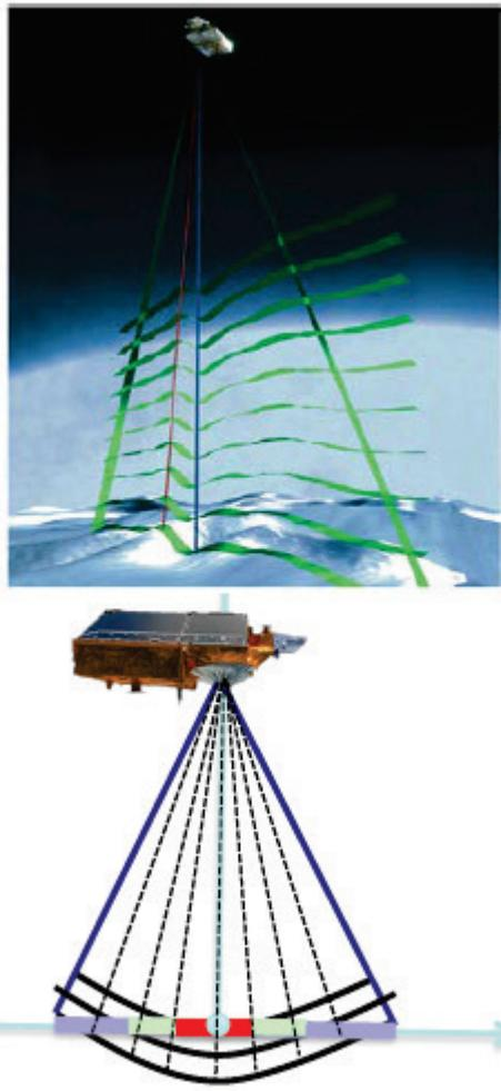
**SAR:** Over sea ice, coherently transmitted echoes are combined, to reduce the illuminated surface area to carry out HR measurements
