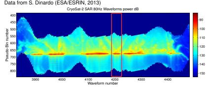
**HR water masks** (e.g., Sentinel-1) + **SAR 80Hz** (or beam steering) = **Optimal set of multilooked waveforms** + reduce CPU cost to a few records
