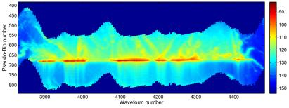
Waveform data  $\ensuremath{\text{reprocessed}}$  at  $80\ensuremath{\text{Hz}}$  (thanks to the presence of 4 bursts per 20\ensuremath{\text{Hz}} cycle)
