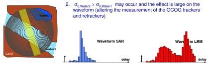
What's new with SAR altimetry for the monitoring of rivers? The "unique" SARIN mode of CrvoSat-2
