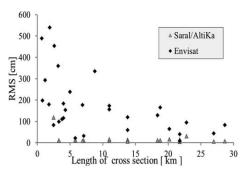
Figure 7 Accuracy with respect to the length of the cross sections.
