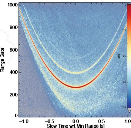
As a radar flies over a fixed point on the Earth, the range (one-way distance) to that point changes from echo to echo. Looking through the instrument's range window at a sequence of pulse echoes, the ground point traces a parabolic trajectory. The total time that the point is “visible” to the radar,  $T_{\text{vis}}$ , depends on how long the point stays in the window. For CS2 & S3,  $T_{\text{vis}}$  is  $\sim 2$  seconds for points near the ground track.
