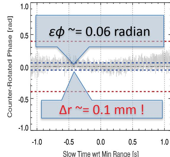
If the FF-SAR calculation employs the maximum possible aperture length ( $T_I = T_{vis}$ ) then it must undo phase changes of the order of 4000 cycles of  $2\pi$ . After doing this, the residual phase error in each pulse echo is about 0.06 radian, only 2 parts per million of the total change in phase occurring across the aperture. (FF-SAR requires a theory of phase more accurate than just the first-order effect. We account for higher-order effects.)
