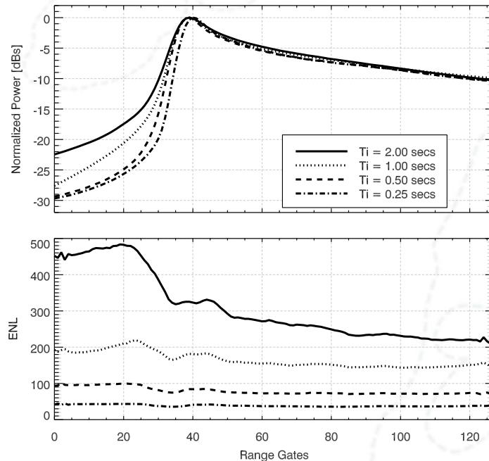
The mean waveform shape depends on the coherent integration time  $T_i$ .  $T_i = 2$  s gives a broad “toe” about 23 dB below peak. Reducing  $T_i$  makes the rise steeper and brings the toe down 30 dB below peak.
