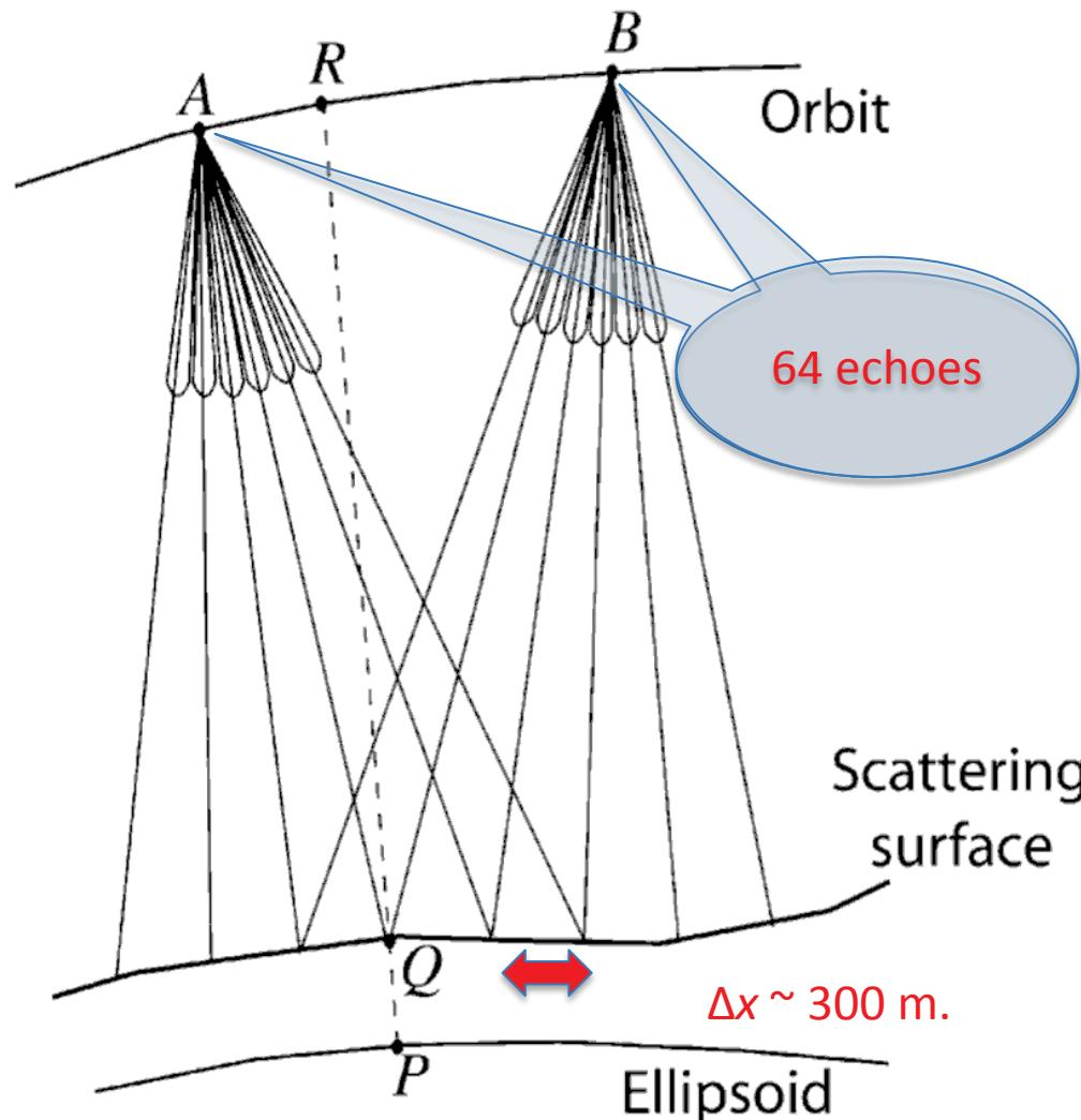
Figure from Wingham et al., 2006, the “multi-looked SAR mode” (also called “Delay/Doppler” [Raney, 1998]) used for Cryosat and Sentinel-3 L1b products applies coherent processing only **intra-burst** (only 64 echoes at a time, 3.52 msec,  $\sim$ 26 m of aperture). Doppler resolution is  $(3.52 \text{ ms})^{-1} = 284 \text{ Hz}$ .
