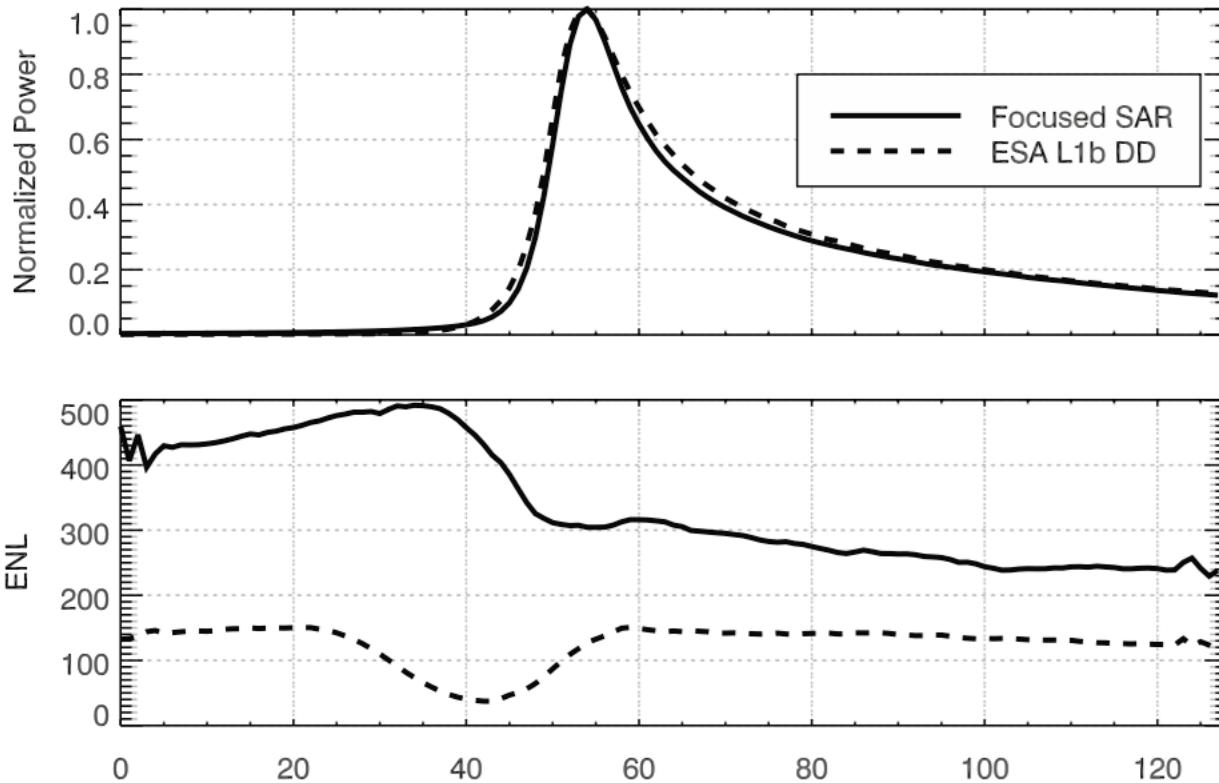
After multi-looking to 20 Hz, so the two can be compared, the mean waveforms of FF-SAR and unfocused D/D SAR (Cryosat L1b) have similar shapes. FF is a little more peaked. The main advantage is that FF ENL is higher than D/D ENL by a factor of 2 to 3, depending on range gate.
