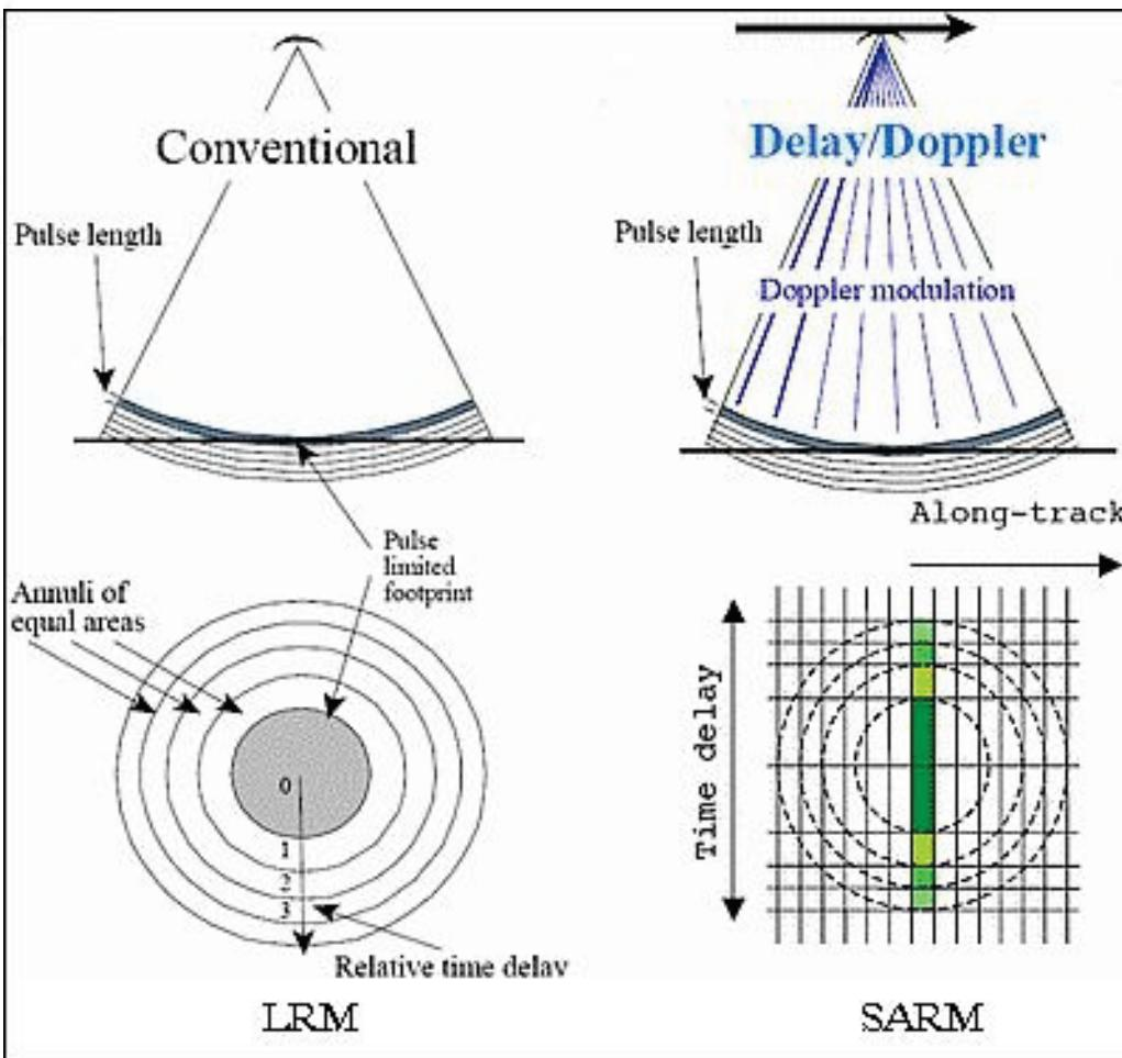
Coherent processing exploits echo-to-echo phase changes to map reflector position to Doppler frequency.
