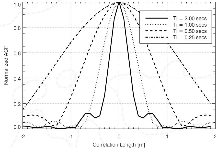
Thus FF-SAR can get statistically independent looks at the ocean every  $\sim 0.5$  m along track, or  $\sim 13,500$  per second. [Almost. The lacunar sampling of closed burst mode causes some small degradation in this, by introducing small side lobes in the along-track PTR.]
