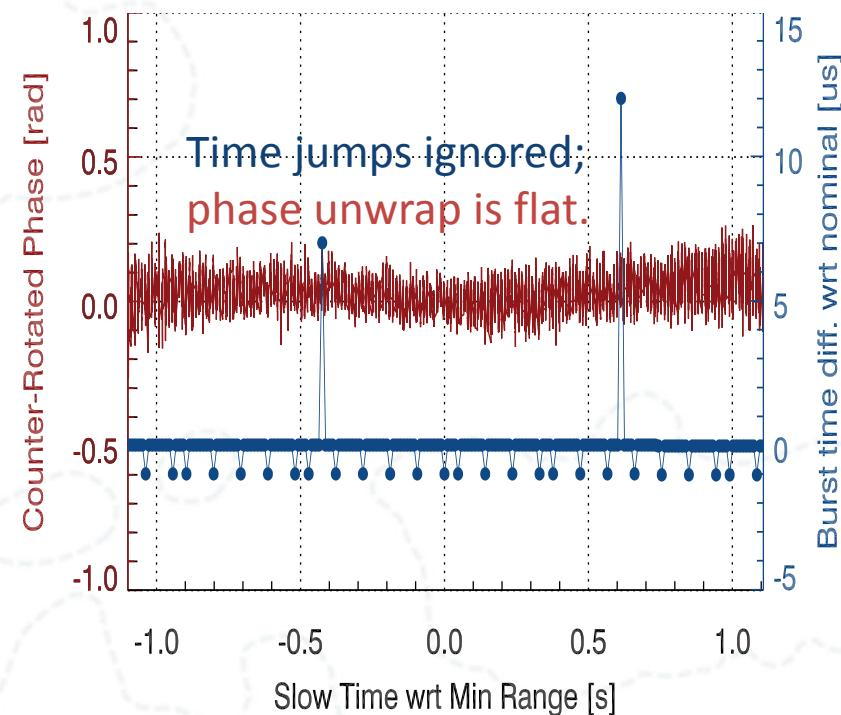
Datation errors of a few microseconds are enough to spoil focus. FF-SAR over a transponder proves that the radar is running steadily even when the datation in the data product shows a jump of a few micro-seconds. To achieve optimal focus we had to correct the datation.
